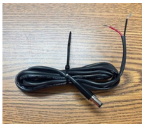
The display power cable connects to truck power 8-30 volt
